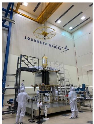
Engineers install Lucy's oxygen propellant tank into the spacecraft structure in a high-bay clean room at Lockheed Martin. Credits: Lockheed Martin Space
